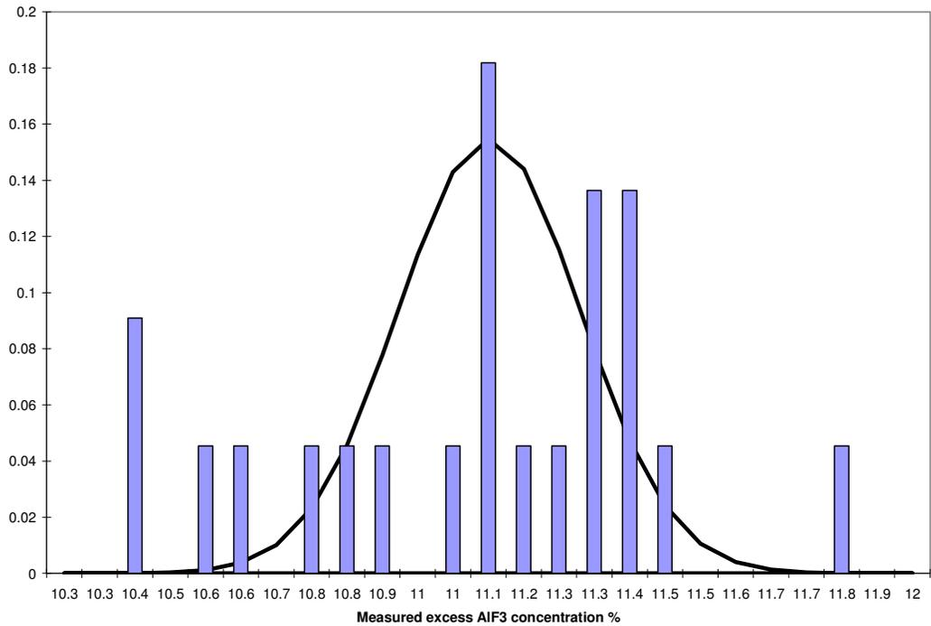
**Figure 5: Distribution of the 22 measured excess AlF<sub>3</sub> concentration**
