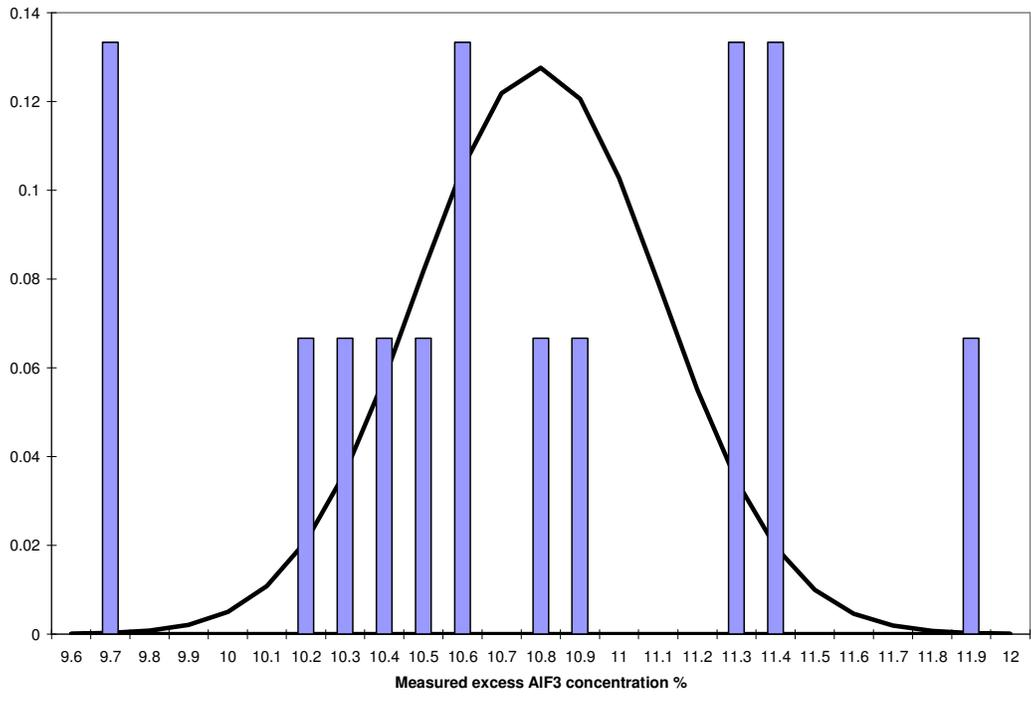
**Figure 1: Distribution of the 15 measured excess AlF<sub>3</sub> concentration**
