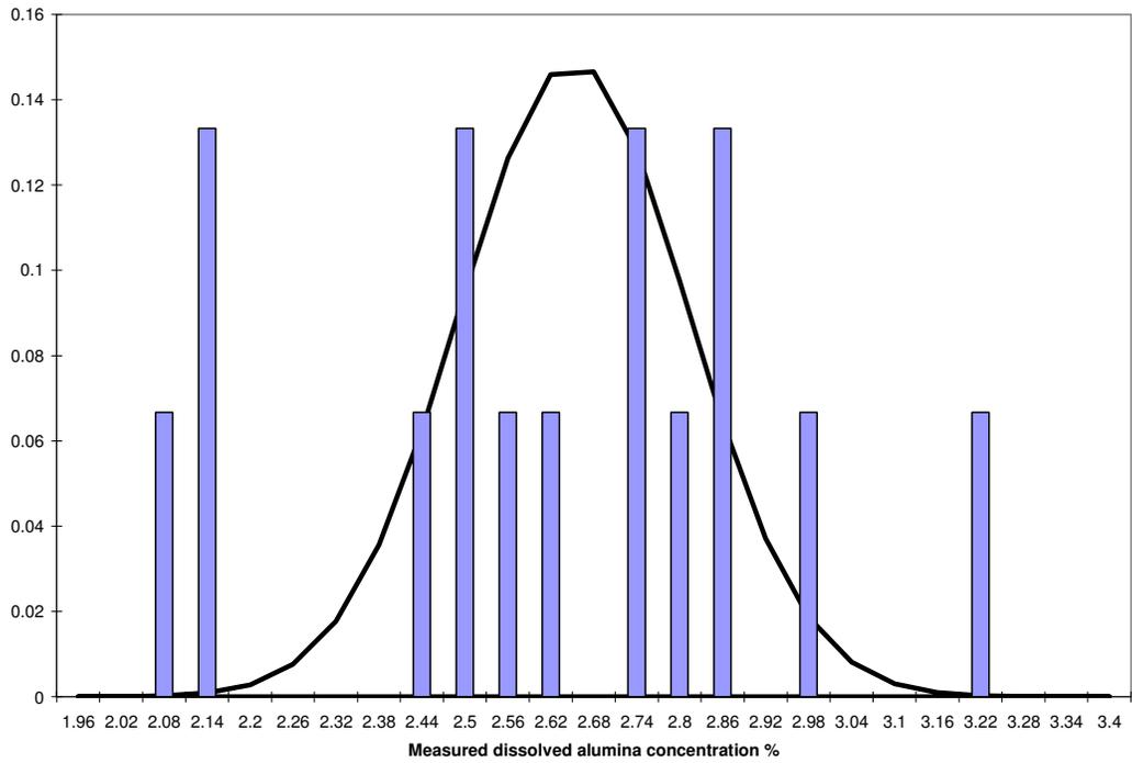
**Figure 3: Distribution of the 15 measured dissolved alumina concentration**
